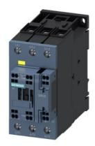
power contactor, AC-3e/AC-3, 51 A, 22 kW / 400 V, 3-pole, 21-33 V AC/DC, 50/60 Hz, with integrated varistor, auxiliary contacts: 1 NC, main circuit: screw terminal, control and auxiliary circuit: spring-loaded terminal, size: S2, F-PLC-IN
