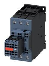
power contactor, AC-3e/AC-3, 51 A, 22 kW / 400 V, 3-pole, 24 V DC, 0.8-1.2\* Us, with integrated varistor, auxiliary contacts: 2 NO + 2 NC, main circuit: screw terminal, control and auxiliary circuit: spring-loaded terminal, size: S2, suitable for PLC outputs, captive auxiliary switch
