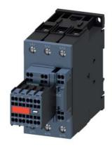
power contactor, AC-3e/AC-3, 51 A, 22 kW / 400 V, 3-pole, 230 V AC, 50/60 Hz, with plugged-in varistor, auxiliary contacts: 2 NO + 2 NC, main circuit: screw terminal, control and auxiliary circuit: spring-loaded terminal, size: S2, captive auxiliary switch
