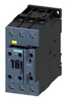
power contactor, AC-3e/AC-3, 51 A, 22 kW / 400 V, 3-pole, 175-280 V AC/DC, 50/60 Hz, with integrated varistor, auxiliary contacts: 1 NC, screw terminal, size: S2, F-PLC-IN
