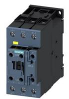
power contactor, AC-3e/AC-3, 51 A, 22 kW / 400 V, 3-pole, 83-150 V AC/DC, 50/60 Hz, with integrated varistor, auxiliary contacts: 1 NC, screw terminal, size: S2, F-PLC-IN
