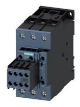
power contactor, AC-3e/AC-3, 51 A, 22 kW / 400 V, 3-pole, 48-80 V AC/DC, 50/60 Hz, with integrated varistor, auxiliary contacts: 2 NO + 2 NC, screw terminal, size: S2, removable auxiliary switch
