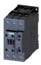
contactor, NEMA version, 25 HP, 460 / 575 V, 3-pole, 208 V AC, 50/60 Hz, auxiliary contacts: 1 NO + 1 NC, screw terminal, size: S2  $\,$
