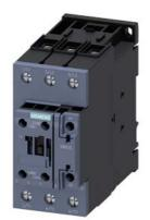
power contactor, AC-3e/AC-3, 51 A, 22 kW / 400 V, 3-pole, 110 V AC, 50 Hz / 120 V, 60 Hz, auxiliary contacts: 1 NO + 1 NC, screw terminal, size: S2, upright mounting position
