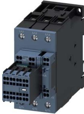
traction contactor, AC-3e/AC-3, 41 A, 18.5 kW / 400 V, 3-pole, 24 V DC, 0.7-1.25\* Us, electronic drive, with integrated varistor, auxiliary contacts: 2 NO + 2 NC, main circuit: screw terminal, control and auxiliary circuit: spring-loaded terminal, size: S2, removable auxiliary switch
