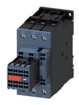
power contactor, AC-3e/AC-3, 41 A, 18.5 kW / 400 V, 3-pole, 24 V DC, 0.8-1.2\* Us, with integrated varistor, auxiliary contacts: 2 NO + 2 NC, main circuit: screw terminal, control and auxiliary circuit: spring-loaded terminal, size: S2, suitable for PLC outputs, captive auxiliary switch
