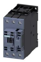
power contactor, AC-3e/AC-3, 41 A, 18.5 kW / 400 V, 3-pole, 230 V AC, 50/60 Hz, auxiliary contacts: 1 NO + 1 NC, main circuit: screw terminal, control and auxiliary circuit: spring-loaded terminal, size: S2
