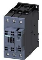
power contactor, AC-3e/AC-3, 41 A, 18.5 kW / 400 V, 3-pole, 110 V AC, 50 Hz, auxiliary contacts: 1 NO + 1 NC, main circuit: screw terminal, control and auxiliary circuit: spring-loaded terminal, size: S2
