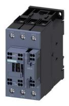
power contactor, AC-3e/AC-3, 41 A, 18.5 kW / 400 V, 3-pole, 24 V AC, 50 Hz, auxiliary contacts: 1 NO + 1 NC, main circuit: screw terminal, control and auxiliary circuit: spring-loaded terminal, size: S2  $\,$
