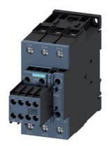
power contactor, AC-3e/AC-3, 41 A, 18.5 kW / 400 V, 3-pole, 175-280 V AC/DC, 50/60 Hz, with integrated varistor, auxiliary contacts: 2 NO + 2 NC, screw terminal, size: S2, removable auxiliary switch
