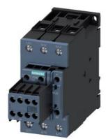
power contactor, AC-3e/AC-3, 41 A, 18.5 kW / 400 V, 3-pole, 20-33 V AC/DC, 50/60 Hz, with integrated varistor, auxiliary contacts: 2 NO + 2 NC, screw terminal, size: S2, removable auxiliary switch
