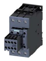
power contactor, AC-3e/AC-3, 41 A, 18.5 kW / 400 V, 3-pole, 230 V AC, 50 Hz, with plugged-in varistor, auxiliary contacts: 2 NO + 2 NC, screw terminal, size: S2, removable auxiliary switch
