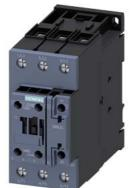
power contactor, AC-3e/AC-3, 41 A, 18.5 kW / 400 V, 3-pole, 48 V AC, 50/60 Hz, auxiliary contacts: 1 NO + 1 NC, screw terminal, size: S2
