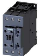
power contactor, AC-3e/AC-3, 41 A, 18.5 kW / 400 V, 3-pole, 24 V AC, 50 Hz, auxiliary contacts: 1 NO + 1 NC, screw terminal, size: S2  $\,$
