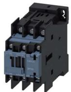
power contactor, AC-3e/AC-3, 38 A, 18.5 kW / 400 V, 3-pole, 48 V DC, auxiliary contacts: 1 NO + 1 NC, ring cable lug connection, size: S0
