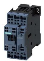
traction contactor, AC-3e/AC-3, 38 A, 18.5 kW / 400 V, 3-pole, 110 V DC, 0.7-1.25\* Us, electronic drive, with integrated varistor, auxiliary contacts: 1 NO + 1 NC, spring-loaded terminal, size: S0
