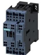
power contactor, AC-3e/AC-3, 38 A, 18.5 kW / 400 V, 3-pole, 110 V DC, auxiliary contacts: 1 NO + 1 NC, spring-loaded terminal, size: S0
