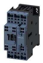
power contactor, AC-3e/AC-3, 38 A, 18.5 kW / 400 V, 3-pole, 208 V AC, 50/60 Hz, auxiliary contacts: 1 NO + 1 NC, spring-loaded terminal, size: S0
