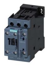
power contactor, AC-3e/AC-3, 38 A, 18.5 kW / 400 V, 3-pole, 24 V DC, with plugged-in varistor, auxiliary contacts: 1 NO + 1 NC, screw terminal, size: S0
