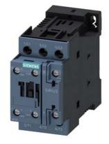
power contactor, AC-3e/AC-3, 38 A, 18.5 kW / 400 V, 3-pole, 230 V DC, auxiliary contacts: 1 NO + 1 NC, screw terminal, size: S0  $\,$
