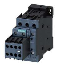
power contactor, AC-3e/AC-3, 38 A, 18.5 kW / 400 V, 3-pole, 24 V DC, auxiliary contacts: 2 NO + 2 NC, screw terminal, size: S0, removable auxiliary switch
