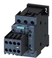
power contactor, AC-3e/AC-3, 38 A, 18.5 kW / 400 V, 3-pole, 24 V AC, 50 Hz, auxiliary contacts: 2 NO + 2 NC, screw terminal, size: S0, removable auxiliary switch
