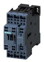
power contactor, AC-3e/AC-3, 32 A, 15 kW / 400 V, 3-pole, 110 V DC, 0.7-1.25  $^{\star}$  Us, with plugged-in varistor, auxiliary contacts: 1 NO + 1 NC, spring-loaded terminal, size: S0, suitable for PLC outputs, not expandable with auxiliary switch
