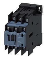
traction contactor, AC-3e/AC-3, 25 A, 11 kW / 400 V, 3-pole, 24 V DC, 0.7-1.25 $^{\star}$  Us, electronic drive, with integrated varistor, auxiliary contacts: 1 NO + 1 NC, ring cable lug connection, size: S0
