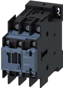
power contactor, AC-3e/AC-3, 25 A, 11 kW / 400 V, 3-pole, 24 V DC, auxiliary contacts: 1 NO + 1 NC, ring cable lug connection, size: S0
