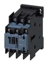
power contactor, AC-3e/AC-3, 25 A, 11 kW / 400 V, 3-pole, 220 V AC, 50 Hz / 240 V, 60 Hz, auxiliary contacts: 1 NO + 1 NC, ring cable lug connection, size: S0
