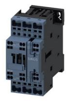
power contactor, AC-3e/AC-3, 25 A, 11 kW / 400 V, 3-pole, 110 V AC, 50 Hz / 120 V, 60 Hz, with plugged-in RC element, auxiliary contacts: 1 NO + 1 NC, spring-loaded terminal, size: S0
