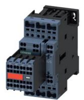
power contactor, AC-3e/AC-3, 25 A, 11 kW / 400 V, 3-pole, 230 V AC, 50/60 Hz, with plugged-in varistor, auxiliary contacts: 2 NO + 2 NC, spring-loaded terminal, size: S0, captive auxiliary switch
