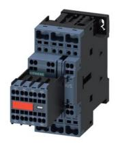
power contactor, AC-3e/AC-3, 25 A, 11 kW / 400 V, 3-pole, 110 V AC, 50 Hz / 120 V, 60 Hz, with plugged-in varistor, auxiliary contacts: 2 NO + 2 NC, spring-loaded terminal, size: S0, captive auxiliary switch
