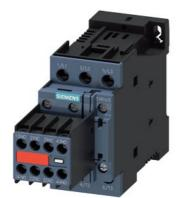
power contactor, AC-3e/AC-3, 25 A, 11 kW / 400 V, 3-pole, 24 V DC, with pluggedin diode combination, auxiliary contacts: 2 NO + 2 NC, screw terminal, size: S0, captive auxiliary switch
