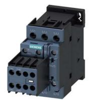
power contactor, AC-3e/AC-3, 25 A, 11 kW / 400 V, 3-pole, 400 V AC, 50 Hz, auxiliary contacts: 2 NO + 2 NC, screw terminal, size: S0, removable auxiliary switch
