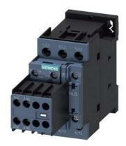
power contactor, AC-3e/AC-3, 25 A, 11 kW / 400 V, 3-pole, 230 V AC, 50 Hz, auxiliary contacts: 2 NO + 2 NC, screw terminal, size: S0, removable auxiliary switch
