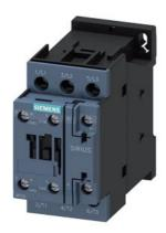
power contactor, AC-3e/AC-3, 25 A, 11 kW / 400 V, 3-pole, 200 V AC, 50 Hz / 200-220 V, 60 Hz, auxiliary contacts: 1 NO + 1 NC, screw terminal, size: S0
