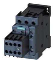
power contactor, AC-3e/AC-3, 25 A, 11 kW / 400 V, 3-pole, 42 V AC, 50 Hz, auxiliary contacts: 2 NO + 2 NC, screw terminal, size: S0, removable auxiliary switch
