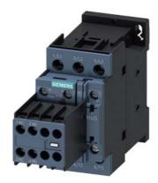
power contactor, AC-3e/AC-3, 25 A, 11 kW / 400 V, 3-pole, 24 V AC, 50/60 Hz, auxiliary contacts: 2 NO + 2 NC, screw terminal, size: S0, removable auxiliary switch
