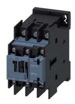
power contactor, AC-3e/AC-3, 17 A, 7.5 kW / 400 V, 3-pole, 200 V AC, 50 Hz / 200-220 V, 60 Hz, auxiliary contacts: 1 NO + 1 NC, ring cable lug connection, size: S0
