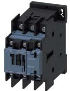
power contactor, AC-3e/AC-3, 17 A, 7.5 kW / 400 V, 3-pole, 110 V AC, 50 Hz / 120 V, 60 Hz, auxiliary contacts: 1 NO + 1 NC, ring cable lug connection, size: S0
