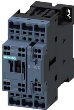
power contactor, AC-3e/AC-3, 17 A, 7.5 kW / 400 V, 3-pole, 200-280 V AC/DC, 50/60 Hz, with integrated varistor, auxiliary contacts: 1 NO + 1 NC, spring-loaded terminal, size: S0
