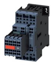
power contactor, AC-3e/AC-3, 17 A, 7.5 kW / 400 V, 3-pole, 230 V AC, 50/60 Hz, with plugged-in varistor, auxiliary contacts: 2 NO + 2 NC, spring-loaded terminal, size: S0, captive auxiliary switch
