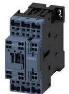
power contactor, AC-3e/AC-3, 17 A, 7.5 kW / 400 V, 3-pole, 24 V DC, auxiliary contacts: 1 NO + 1 NC, spring-loaded terminal, size: S0, communication-capable
