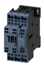
power contactor, AC-3e/AC-3, 17 A, 7.5 kW / 400 V, 3-pole, 230 V AC, 50 Hz, auxiliary contacts: 1 NO + 1 NC, spring-loaded terminal, size: S0, upright mounting position
