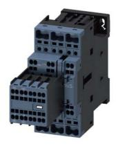
power contactor, AC-3e/AC-3, 17 A, 7.5 kW / 400 V, 3-pole, 230 V AC, 50/60 Hz, auxiliary contacts: 2 NO + 2 NC, spring-loaded terminal, size: S0, removable auxiliary switch
