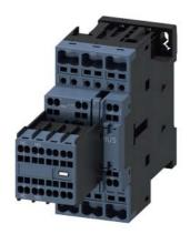
power contactor, AC-3e/AC-3, 17 A, 7.5 kW / 400 V, 3-pole, 110 V AC, 50/60 Hz, auxiliary contacts: 2 NO + 2 NC, spring-loaded terminal, size: S0, removable auxiliary switch
