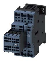
power contactor, AC-3e/AC-3, 17 A, 7.5 kW / 400 V, 3-pole, 24 V AC, 50 Hz, auxiliary contacts: 2 NO + 2 NC, spring-loaded terminal, size: S0, removable auxiliary switch
