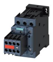
power contactor, AC-3e/AC-3, 17 A, 7.5 kW / 400 V, 3-pole, 24 V DC, with plugged-in diode combination, auxiliary contacts: 2 NO + 2 NC, screw terminal, size: S0, captive auxiliary switch
