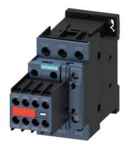
power contactor, AC-3e/AC-3, 17 A, 7.5 kW / 400 V, 3-pole, 230 V AC, 50/60 Hz, with plugged-in varistor, auxiliary contacts: 2 NO + 2 NC, screw terminal, size: S0, captive auxiliary switch
